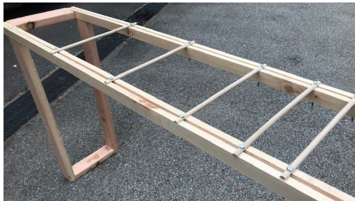
Fig. 4: The experimental rig is made of wood and has adjustable rung spacing.
